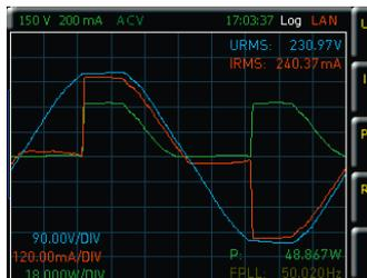
Waveform: load with phase-angle control
