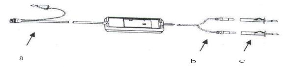
a. Output Cable The BNC output connector and an auxiliary grounding terminal are connected to the oscilloscope.
