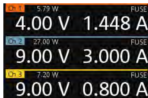
Figure 5-11: Fuse switched on for the respective channel
