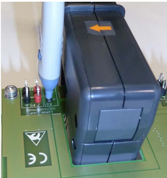
Figure 2-1: R&S RT-ZC10 and R&S RT-ZD30 differential probe at large loop
