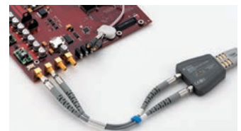
N5444A InfiniiMax III 2.92-mm SMA with N5448A SMA flex cable connected to a SMA connector on the board
