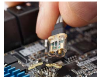
N2848A QuickTip head with N2849A QuickTip tips
