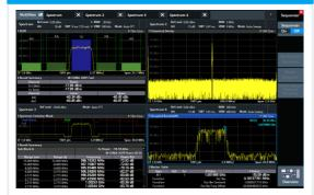
Configure your result windows the way you want. Display multiple measurement channels at once. Sequential channel updating allows e.g. parallel measurement of the spectrum, spectrogram and analog demodulation together with I/Q analysis.
