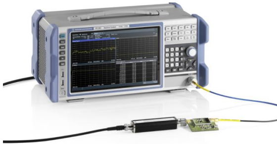
Measure the noise figure and gain of amplifiers using an R&S®FPL1000 with the R&S®FPL1-K30 option and a noise source
