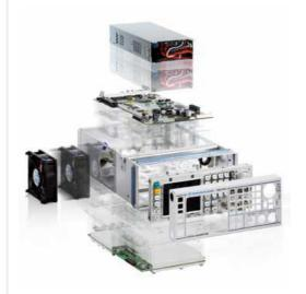
A minimum of modules in the R&S°SMC100A means high reliability and easy servicing.
