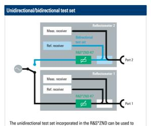
test passive components such as filters, connectors and antennas.
