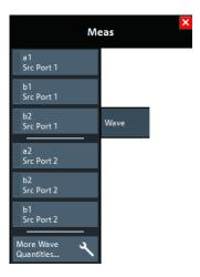
The "More Wave Quantities..." button opens the More Wave Quantities dialog which allows to select an arbitrary wave quantity, e.g. for different source ports or higher port numbers.
