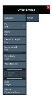
The "Fixture Compensation..." button opens the Fixture Compensation Dialog.
