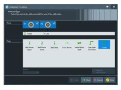
The calibration wizard provides an overview of the possible calibration methods for easy selection.
