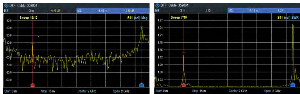
Figure 7-5: Distance to fault measurement
