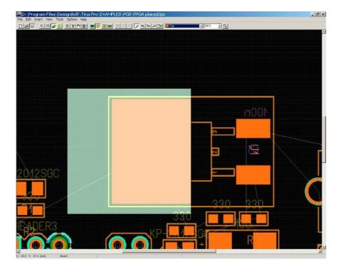
When you double click on the area, you can enter the parameters exactly. Do not forget to check the shape type and select Assigned net 2.5V. Normally, copper pour creates voids where there are tracks or pads except for the Assigned net. (See Options/Design Parameters). The other shape type is the copper fill area which is solid.
