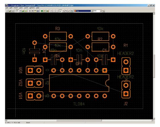
Press F4 to reach the Net Editor and set net routing width. First, click on "Modify all" and enter 12.5 into "Track width" field. Then select power nets (Ground, VCC, -VCC) and set their width to 25mil.
