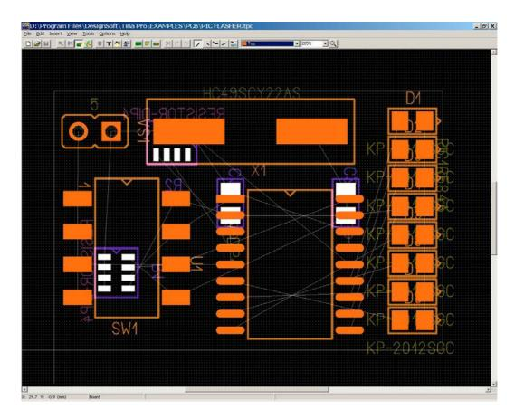
In order to decrease route length, swap R1 pins connected to SW1. Pin swapping is allowable if identically functioning pins are to be exchanged, such as pins of resistors, capacitors, etc. Click on the Pinswap button on the toolbar to pick up the tool, click on pad 1 of R1 (the upper right), and-finally-pad 4 of R1. The following window should come up:
