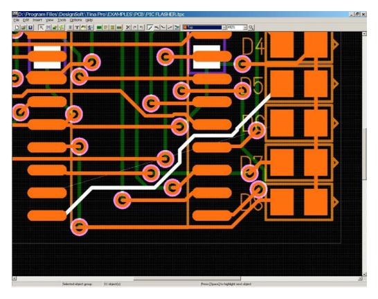
Now press F4 to invoke the net editor. Disable N00012, the previously removed connection. This will prevent the autorouter from reconnecting the net. Leave N00013 routing enabled.
