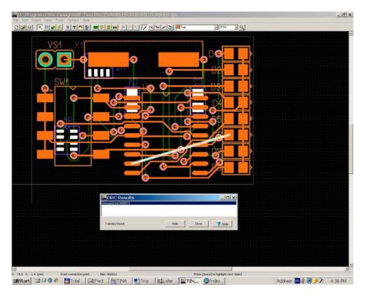
In order to fully route the board, we can use the manual route modes to make space for the unconnected tracks or delete crossing tracks and reroute them in a different order. Working in manual route, you can direct routing wherever necessary. You can move existing segments of tracks, remove segments, or create new segments.
