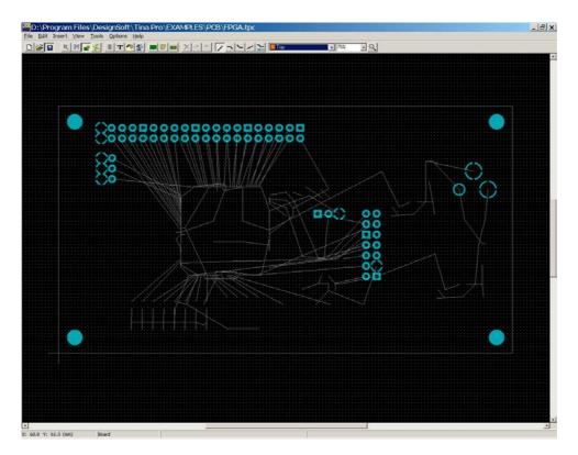
You can now see all of the connections to the ground plane. You can do the same thing for the power plane: Option/Layer settings, uncheck Ground and check Power.
