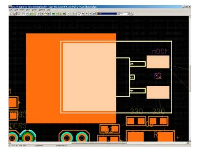
Finally, repeat these operations for the other voltage regulator and save your design. Note, you can find this state of the design if you open \Examples\PCB\FPGA placed.TSC.
