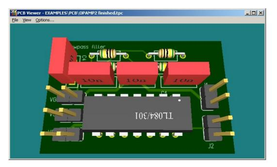
You can rotate the 3D model to any direction by clicking with the mouse at any point. Hold down the left button and move the mouse to shift the viewpoint. You can also move the "camera" forward or backward to set a large view showing the complete PCB or to zoom in for more details. Use the right mouse button for this operation.
