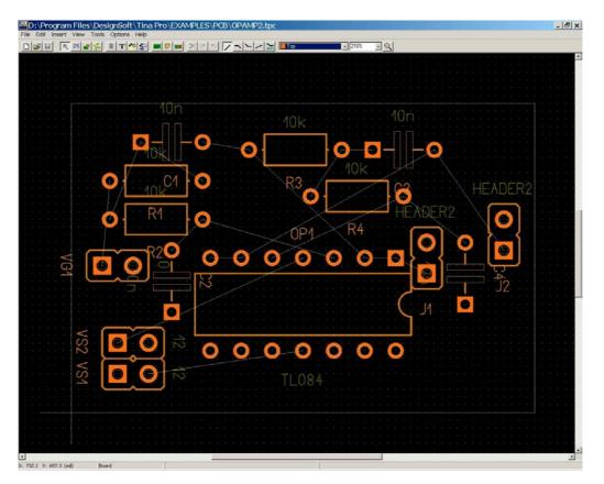
While all the parts and nets are placed, we need to adjust their positions for good placement and easier routing. Click and drag the parts to the position as shown on the figure below. (Find "opamp2 placed.tpc" to check your results.)
