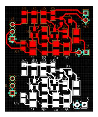
Press F5.You can now do the rest of the routing with the Autorouting tool and/or some manual editing. The result should be like that shown in the *Stereo microphone preamp routed.TPC* file.
