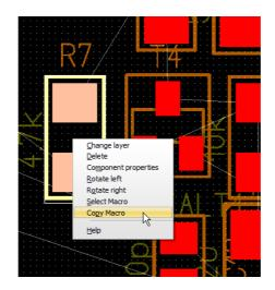
The program will automatically place and route the parts belonging to the U2 macro. The initial alignment is based on the position you selected for the resistor R1 in the copy-paste operation, but you can move this component group to a different place on the board if needed.
