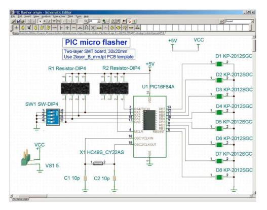
The schematic is PCB-ready-as you can verify by pressing the 2D/3D button, every part has a surface mount device (SMD) physical representation. Now, before we start the PCB wizard, click Tools/Footprint Name Editor... to check the footprints list.
