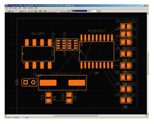
The components are placed in the close proximity to minimize the connection lengths, in a topology similar to that of the schematic, while still respecting the design rule settings. However convenient the result may be for autorouting, the designer usually has to make adjustments to the component layout to satisfy electrical, mechanical and other characteristics. Some of the considerations are—
