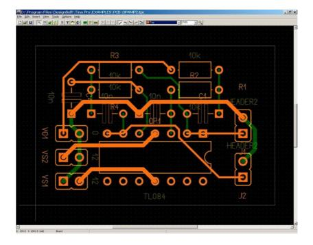
To automatically route the PCB, press the F5 button or select "Autoroute board" command from the Tools menu. The following screen will appear:
