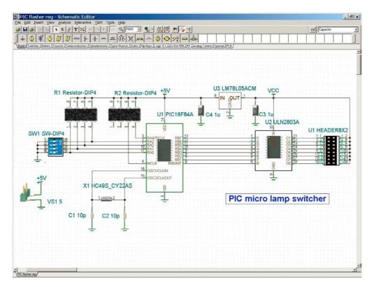
As the electric type of U3 pin 1 (OUT) is defined to be an output and is connected to the power pins of U1 and U2, you will encounter ERC errors when you call PCB Wizard or perform an ERC. But knowing that U2 is the power source for the ICs, we can safely disregard this error.
