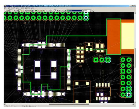
Plane layers are negative layers, so only the isolating "moats" can be seen on the screen. Before beginning other tasks, you should assign the 2.5V net to its split area. Double click on the shape, select the 2.5V net, and click OK.
