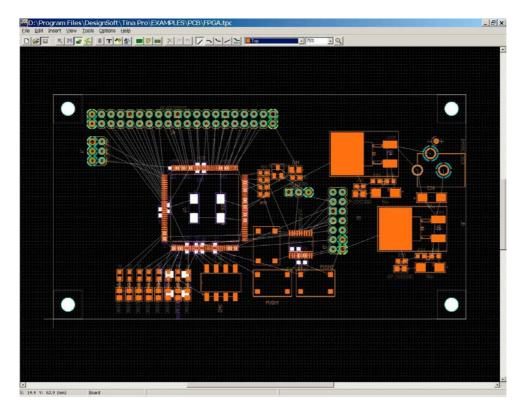
The silkscreen is a bit messy, but we will deal with that later. In fact, during routing the silkscreen can get in the way, so you may turn off the silkscreen and assembly layers now, just as you did earlier to suppress the two inner layers.
