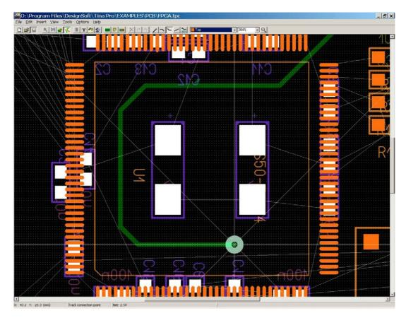
Connect all the power pins of the FPGA, then the pads of filter and decoupling capacitors; set the track width to 0.4mm. Now make the power track 2mm wide as shown below by double clicking on the track.
