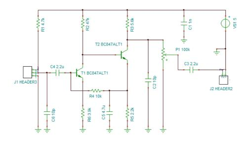
This circuit is a mono-microphone preamplifier with simplified external connections. Turn this circuit into a schematic macro subcircuit in order to add one more channel to the amplifier.
