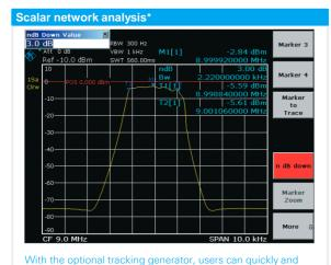
easily measure frequency response, filters and attenuation.
