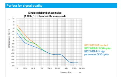
Thanks to its innovative synthesizer design, the R&S $^SMB100B$  has very low SSB phase and wideband noise and excellent suppression of nonharmonic signal components
