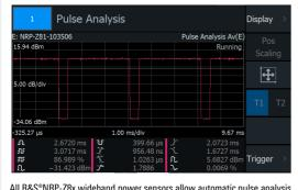
All R&S\*NRP-Z8x wideband power sensors allow automatic pulse analysis. Up to 12 of 18 user-selected pulse parameters can be displayed in addition to the measurement trace.
