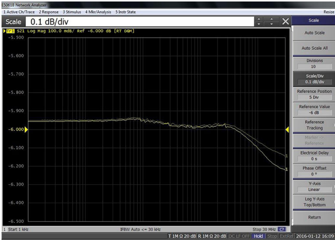
Figure 57: The 6dB splitter is accurate to within 0.25dB across the full frequency range of the instrument.
