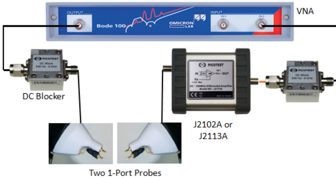
Figure 41: Test setup for measuring the in-circuit output impedance using two 1-Port PDN Probes (P2100A). The J2102A has been replaced by the J2102B.
