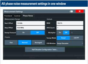
All settings for phase noise measurements (e.g. measurement range, average
