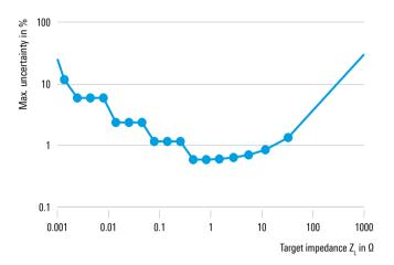
Impedance accuracy for the low impedance setup calculated from R&S $^{\circ}$ ZNL calibrated specified transmission accuracy and valid for the entire spectrum. Data between -65 dB and -90 dB is extrapolated.
