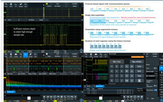
Analyze past acquisitions before the error occurred. The history function ensures that previous waveforms stored in memory can always be accessed. A trigger timestamp allows time correlation. You can view all saved signals and analyze them with tools such as zoom, measurement, math and spectrum analysis functions.
