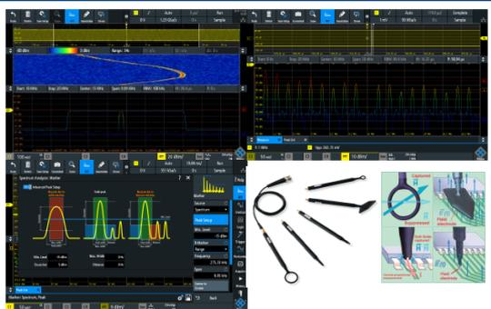
Difficult-to-find faults often result from the interaction between time and frequency signals. The R&S®RTx-K37 spectrum analysis and spectrogram option quickly finds such errors. Parameters such as center frequency and resolution bandwidth can be easily adapted to the specific measurement task. The oscilloscope automatically selects the relevant time domain settings.
