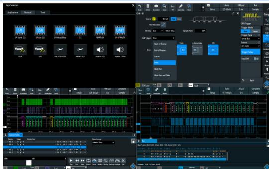
Protocols such as I<sup>2</sup>C, SPI and CAN/LIN frequently transfer control messages between integrated circuits. The R&S®RTB2000, R&S®RTM3000 and R&S®RTA4000 offer versatile options for protocol-specific triggering and decoding of serial interfaces.
