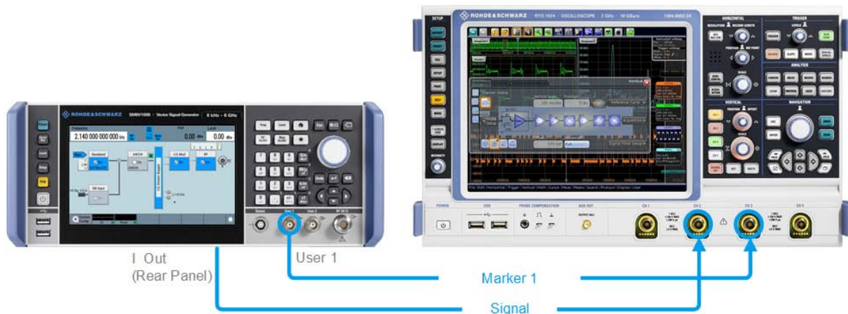
Figure 6-7: Simplified representation of a test setup for signal monitoring**
