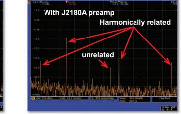
Conducted EMI measurements of a Wireless Power Transmitter with and without the J2180A preamp.
