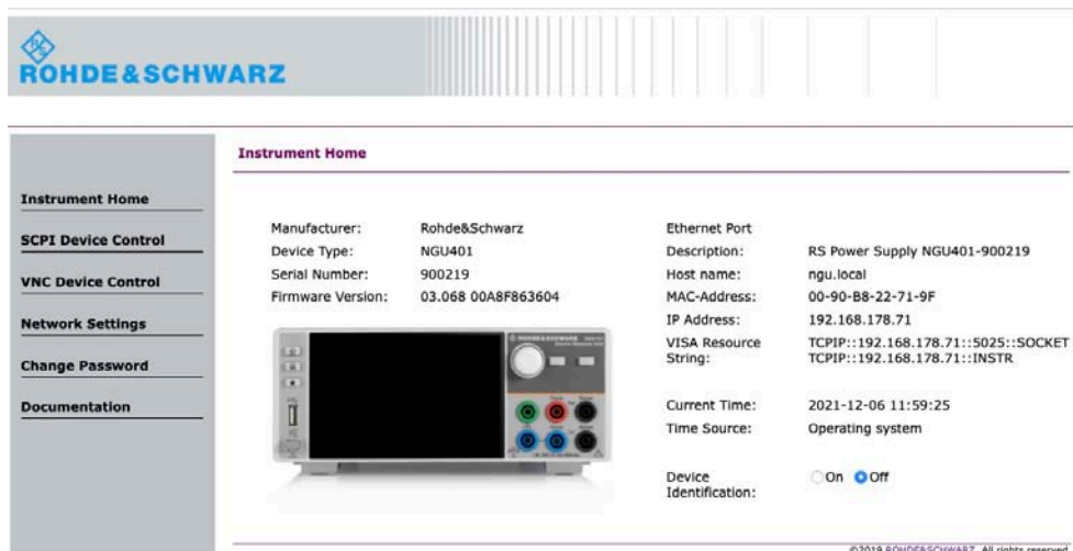
Figure 6-67: Instrument home webpage of a power supply model
