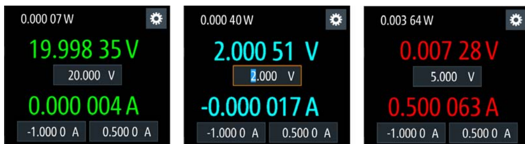
Figure 5-3: Color coding of difference operating conditions
