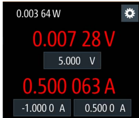
Figure 6-2: Output of R&S NGU in CC mode
