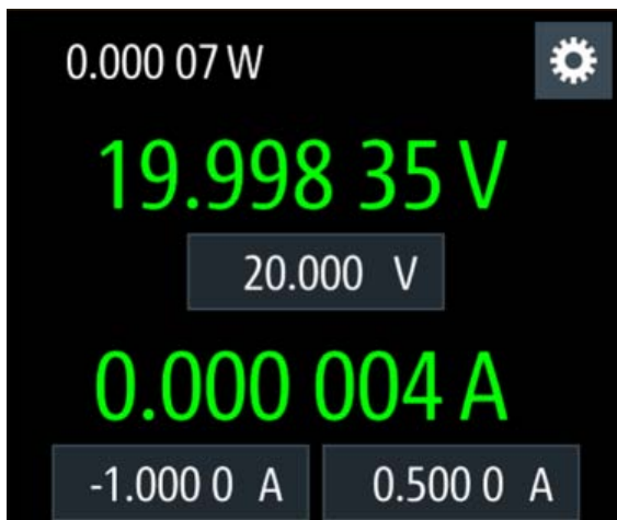
Figure 6-1: Voltage and current settings in the instrument
