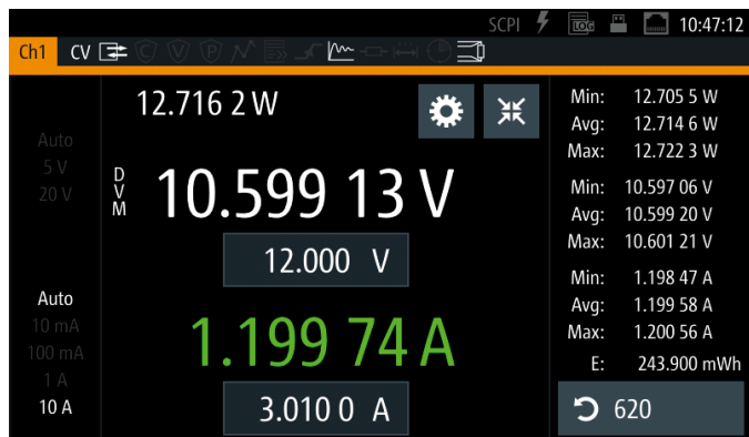
DVM display on an R&S®NGM200 power supply.
