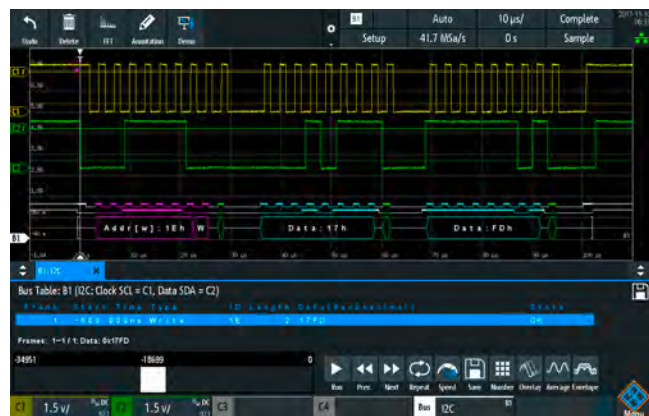
Decoded I2C signal with analog waveforms on the R&S®RTM3000.
