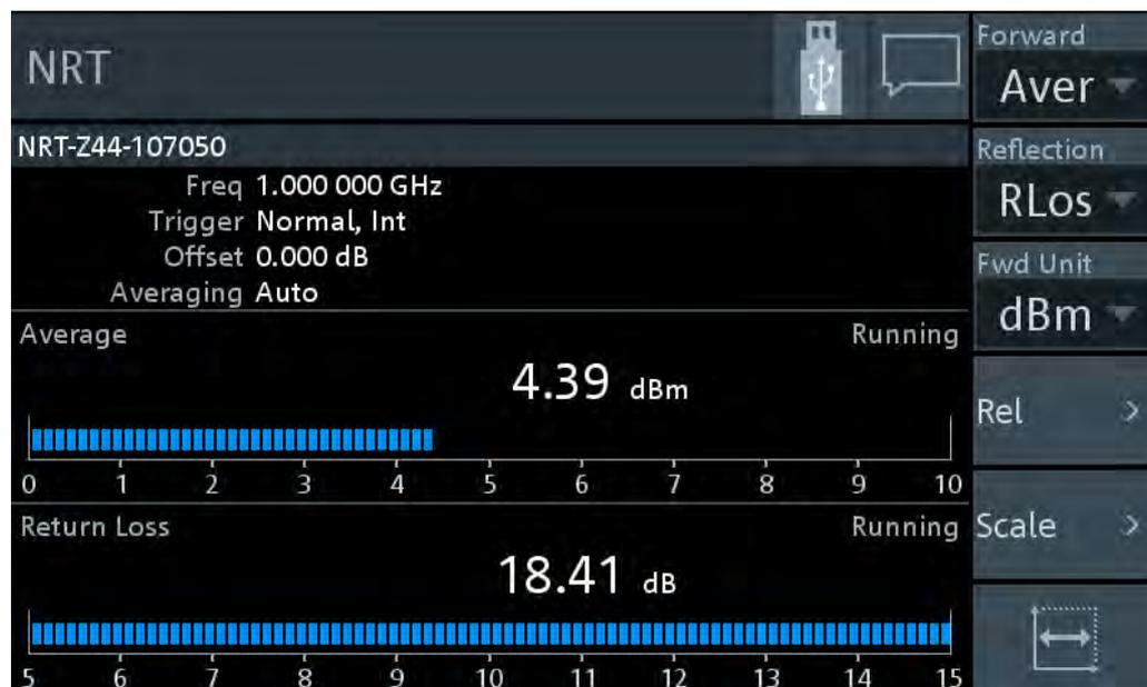
The R&S NRT2 displays the forward and reverse power simultaneously. One scalar value for the selected **Forward** measurement, and one scalar value for the **Reflection** measurement.
