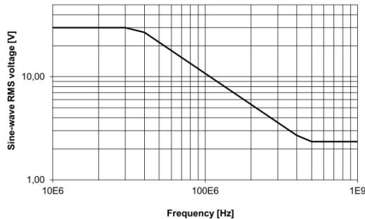
*R&S®RT-Z1M maximum rated sine-wave root mean square input voltage versus frequency***R&S®ProbeMeter**
