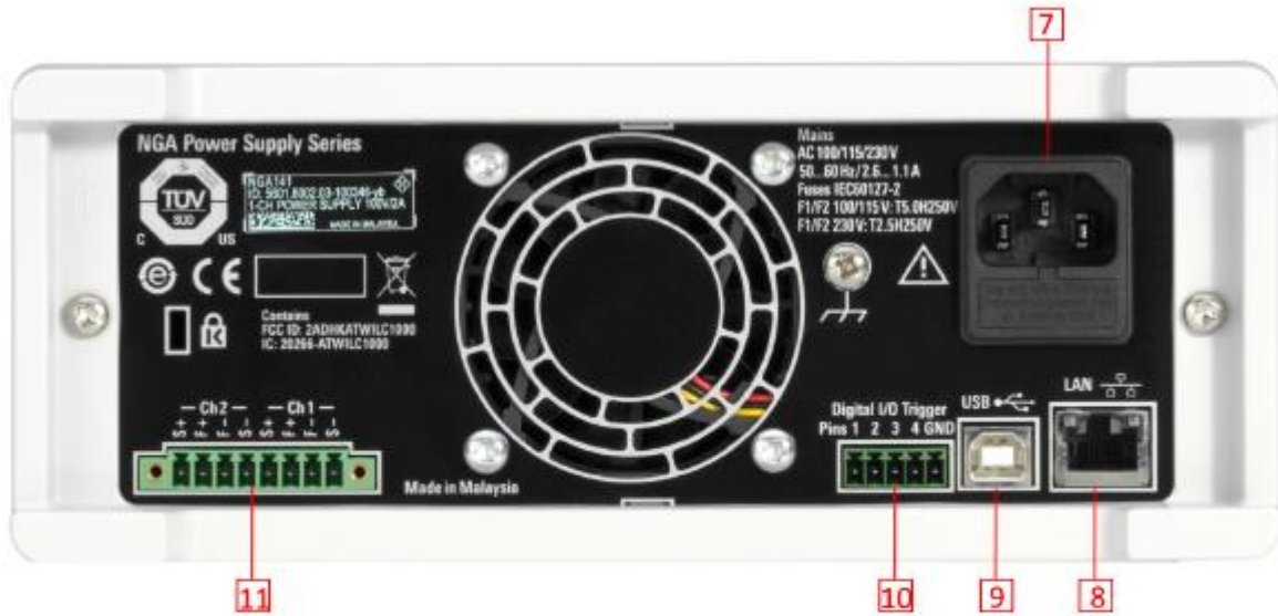
Figure 4-2: Rear panel of R&S NGA100
