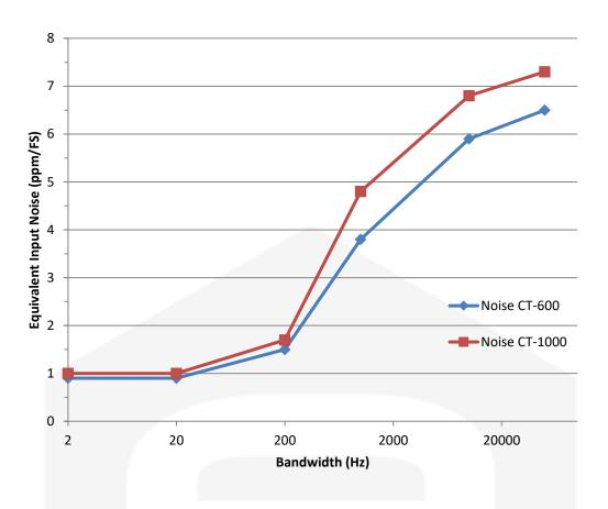
Figure 12: Equivalent input noise graph (typical values)
