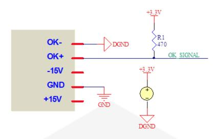
Figure 6: OUT OK signals connections as digital interfacing to +3.3V
