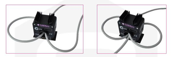
Figure 11: primary full-scale current scaled by a factor 2 (2 primary turns - left) and scaled by 3 (3 primary turns - right)
