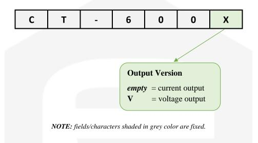
The **CT-1000** current transducers have also two different versions differing by the secondary output signal types (current or voltage). The ordering code is formatted as follows:
