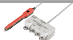
PINCHER PROBE L2001 Cable length 73 cm (2.40 ft), DC to 8 MHz, impedance characteristics of 50 Ω, 4-terminal pair configuration, tip electrode spacing: 0.3 (0.01 in) to 6 mm (0.24 in)
