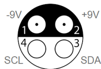
Probe's power supply pin assignment "cable view"
