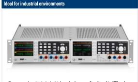
Power supply units in industrial production are often found in 19" racks. All R&S®NGC100 models can be integrated into 19" racks with the R&S®HZC95 rackmount adapters.
