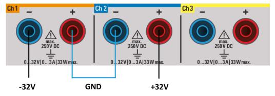
Figure 5-3: Setup to generate -32 V and +32 V
