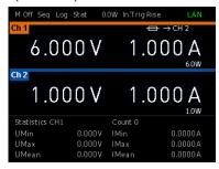
Figure 5-7: Linking of channel 2 to channel 1
