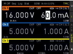
Figure 5-2: Voltage and current settings in the instrument
