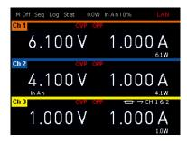
Figure 5-9: Indicator of OVP/OPP when tripped
