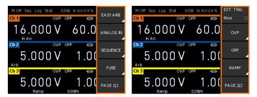
Figure 3-13: Example of a menu selection (highlighted)
