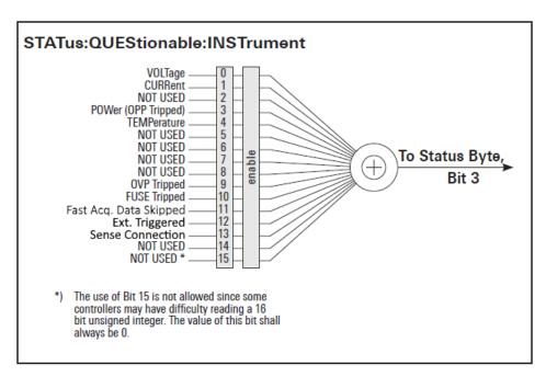
Figure 8-9: Structure of the status: QUEStionable: INSTrument register
