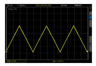
Figure 5-23: Arbitrary waveform example
