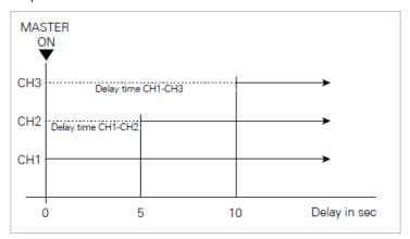
Figure 5-13: Example for R&S NGC103(-G) model sequencing
