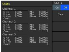
Figure 3-10: Statistic display of a R&S NGC101(-G) and R&S NGC103(-G) model
