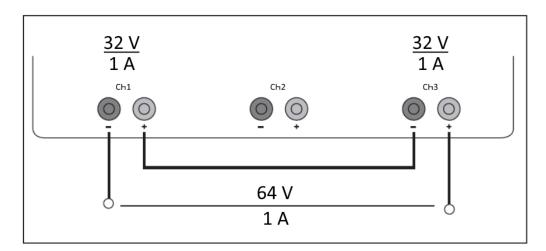
Figure 13-1: Example of series connection
