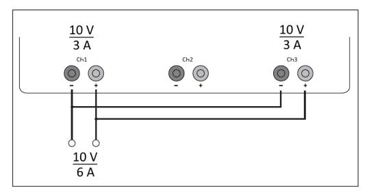
Figure 13-2: Example of parallel connection
