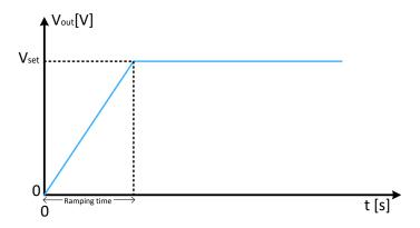
Figure 5-27: Ramping voltage output
