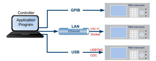
Figure 8-1: Supported remote connections
