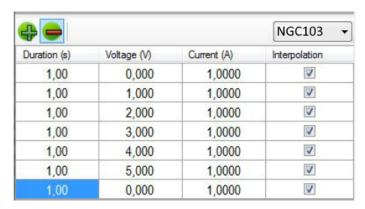
Figure 5-25: Arbitrary-editor example (excerpt) R&S HMExplorer software
