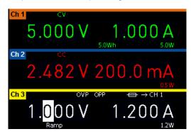
Figure 3-11: Color coding of difference operating conditions
