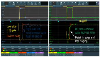
CMRR suppression critical for high-side (HS) gate measurements
