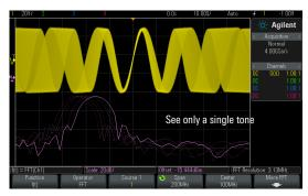
Keysight 3000X FFT: Limited memory results in poor resolution. Slow update misses significant signal details.
