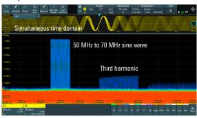
MXO 3 spectrum displays time and frequency simultaneously. See all details instantly with fast updates.
