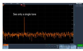
Tektronix MD03 spectrum: Time not visible simultaneously. Slow update misses significant signal details.
