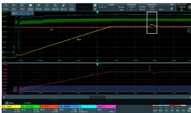
Fig. 5: Startup of the converter and irregular control effects
