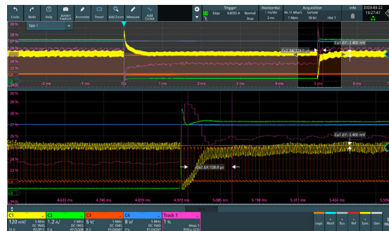
Fig. 3: Load transient setup of a step-down converter
