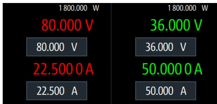
Figure 5-3: Output of R&S NGT3600 in CC and CV modes
