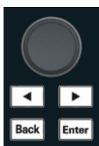
Navigation in the menu and setting of values can be done via rotary knob, arrow keys, [Back] key and [Enter] key.
