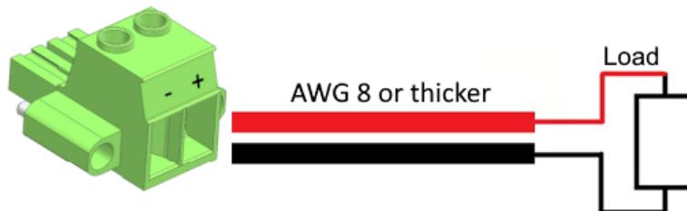
*Figure 3-7: Connection to load*
