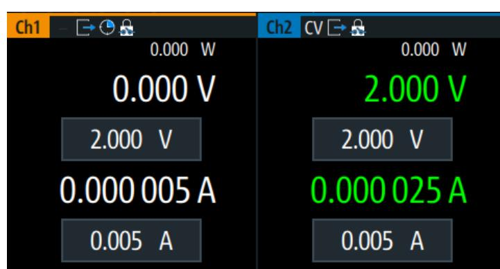
Figure 5-8: Delay function activated in channel 1
