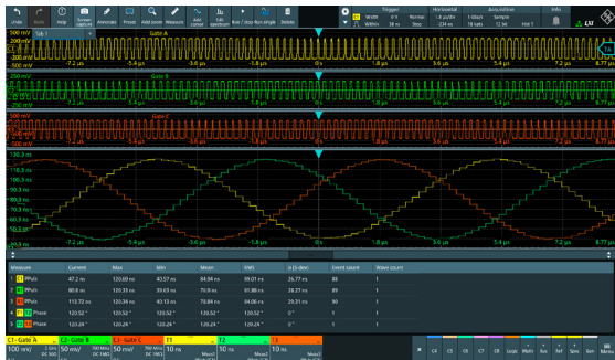
MXO with track function can visualize PWM into traces for analysis
