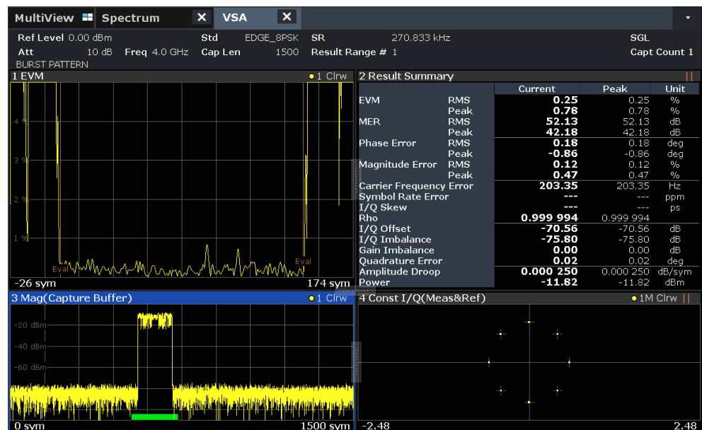
Figure 10-11: Solution: Result Summary with correct evaluation range setting
