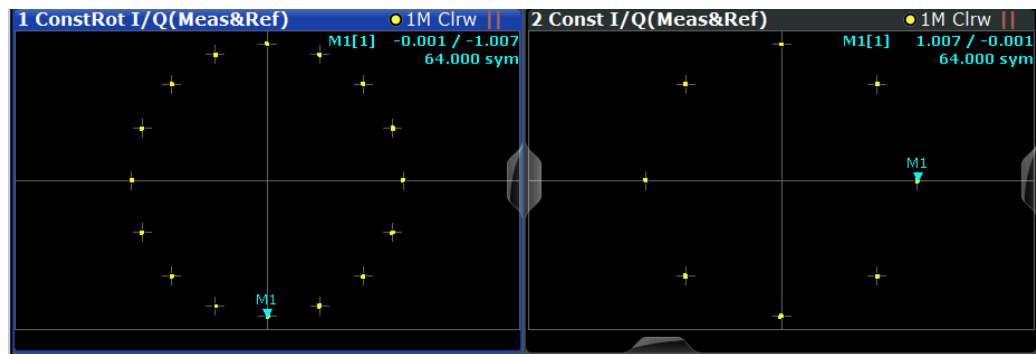
Figure 3-5: Constellation I/Q (Rotated) result display vs. common Constellation I/Q for 3π/8-8PSK modulation
