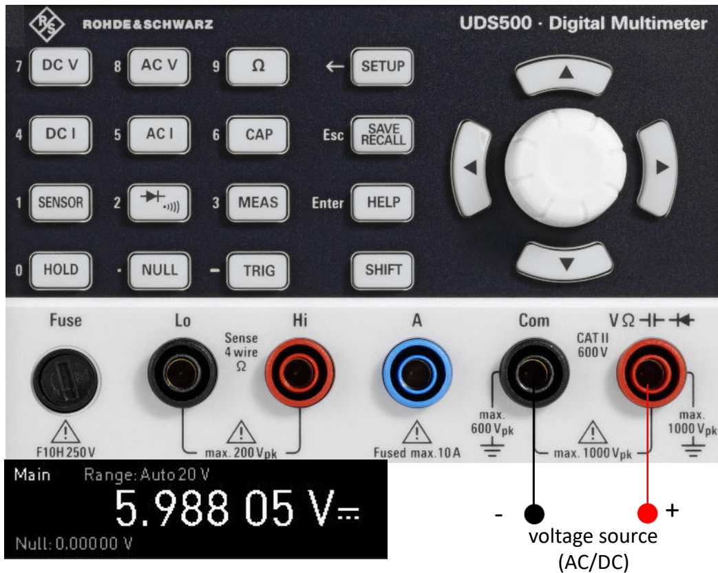
Figure 5-1: Connections for AC/DC voltage measurement
