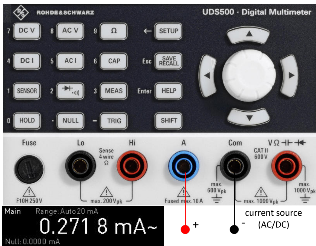
Figure 5-3: Connections for AC/DC current measurement
