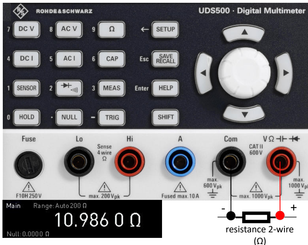
Figure 5-5: Connections for two-wire resistance measurement
