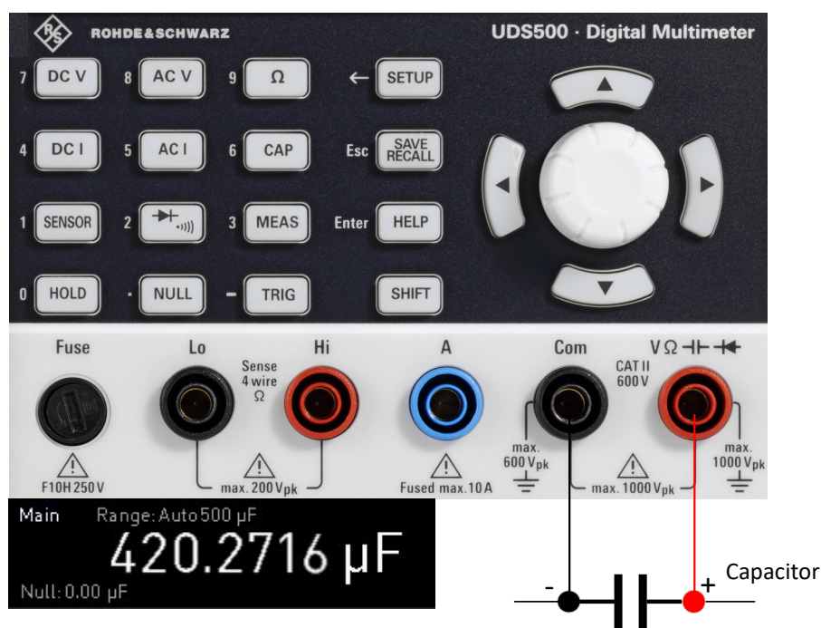
Figure 5-4: Connections for capacitance measurement
