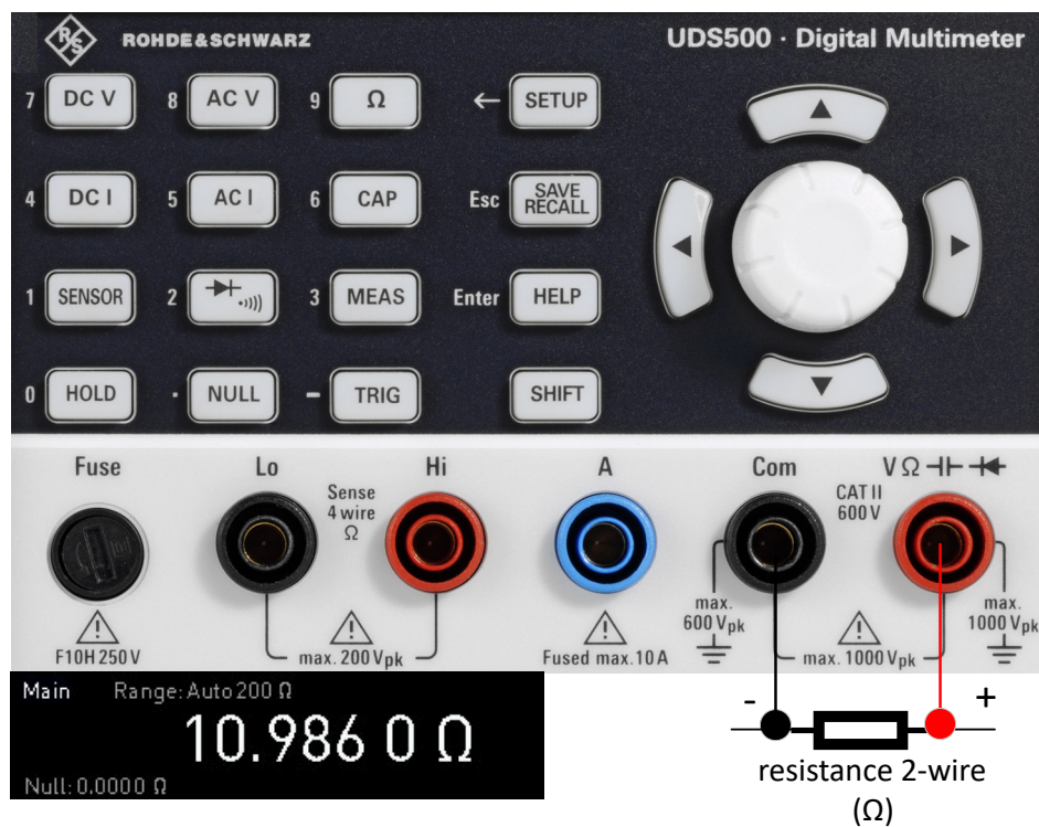
Figure 5-2: Connections for two-wire resistance measurement
