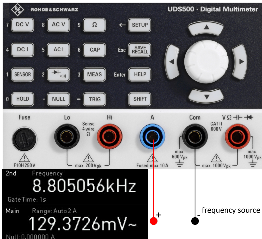
Figure 5-1: Connections for frequency measurement
