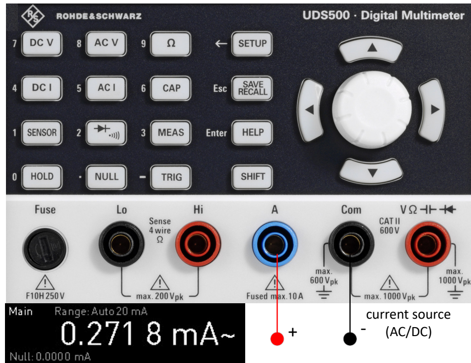
Figure 3-7: Connections for AC/DC current measurement
