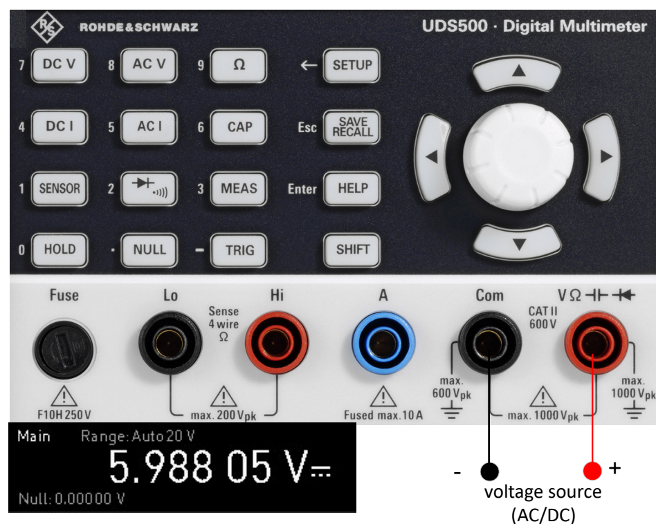
Figure 3-5: Connections for AC/DC voltage measurement
