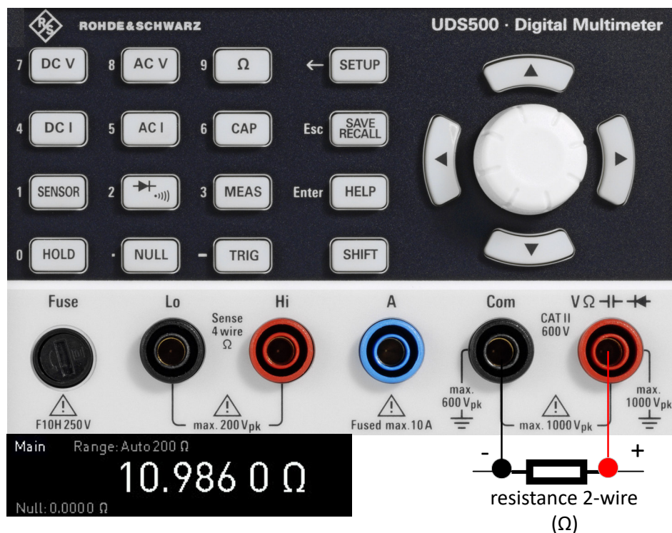
Figure 3-9: Connections for two-wire resistance measurement
